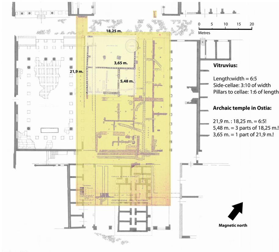
Fig. 10. The Late Archaic temple in Ostia follows three Vitruvian principles. The plan is based on The Belvedere Temple in Orvieto (Colonna 1985, fig. 4.7), plan by I. Gismondi (Scavi di Ostia I, fig. 21 & Archivio Disegni B481), plan by I. Gismondi & O. Visca (I, Pianta Generale).
